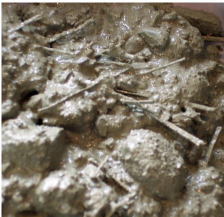
TECHNOFIBER® in fresh concrete
