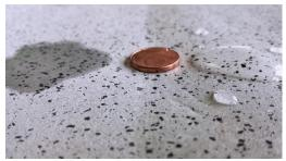
Left: unprotected - water penetrates the surface Right: protected with **COLORFRESH® intensiv** - water is repelled
