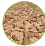
Medium exposure. Exposure depth approx. 2.5 mm
