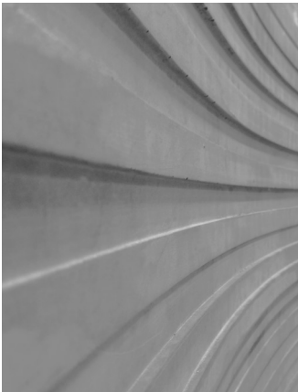
The photo above shows an example of a concrete surface produced in a structured formliner by using WABICON HP as mould release agent.
